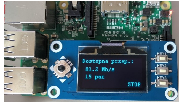
Fig. 3. Path state measurer during local, manual measurement. Available throughput ("Dostępna przepustowość" in Polish) is 81.2 Mbps, packet train was set to 15 pairs. The right, down button stops measurements.
