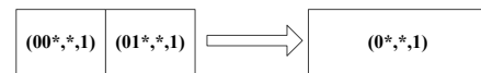
Fig. 2. Entry (00*, *, 1) and Entry (01*, *, 1) are left-right adjacent and can be merged into one entry (0*, *, 1) .
