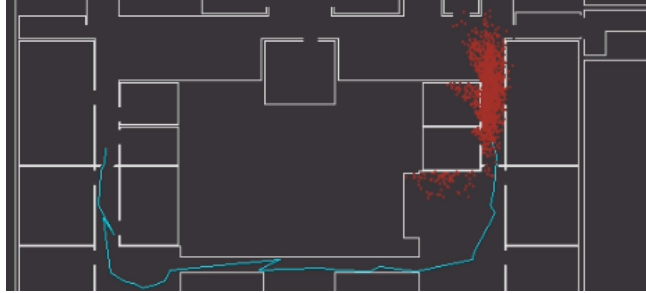
Fig. 6. Example run of a particle filter implemented using the PerPos middleware. Red dots indicate particle positions, the blue line indicates the evaluated trace, and white lines indicate walls.
