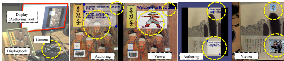
Fig. 7. Snapshots of the multi-layer authoring tool: (from the left) environmental setup, mapping a figure and a video to two layers, example of another page authoring
