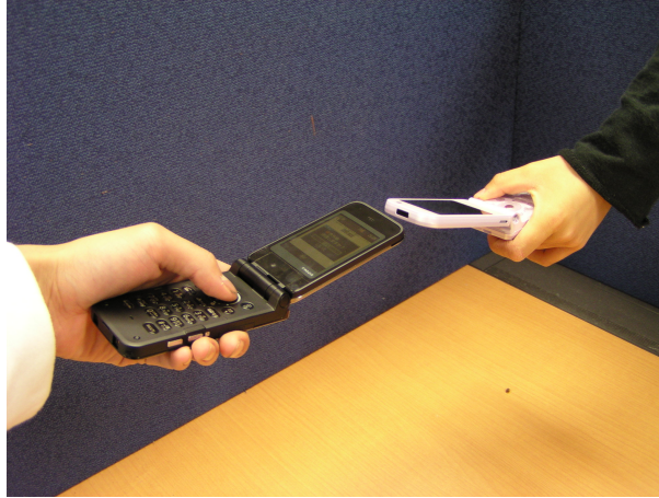
Fig. 3. An infrared communication between mobile phones
