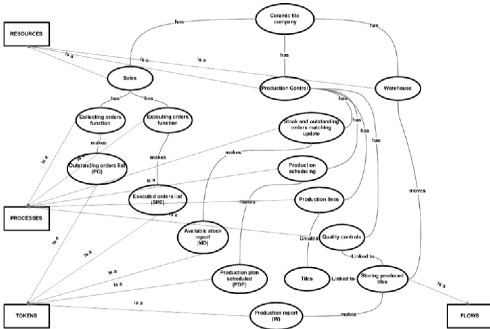
Fig. 4. Tile enterprise reference FDM model.
