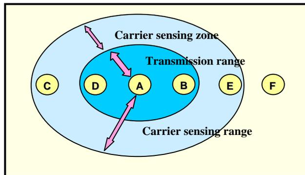
**Fig. 1** Two disjoint areas of carrier sensing zone and transmission range, both of which constitute the carrier sensing range for node A. We assume that node A is a sender and node B is a receiver and transmission range from a frame transmitting source is one hop and carrier sensing range is two hops. Then node C and E is said to be in carrier sensing zone of the sender side.
