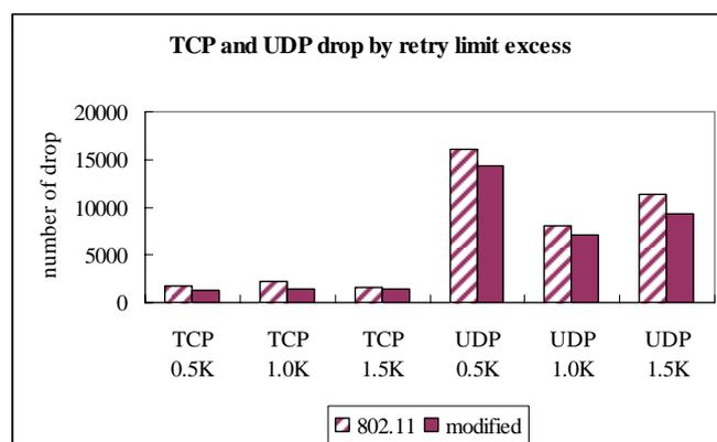
**Fig. 8** TCP and UDP drop by limit excess
