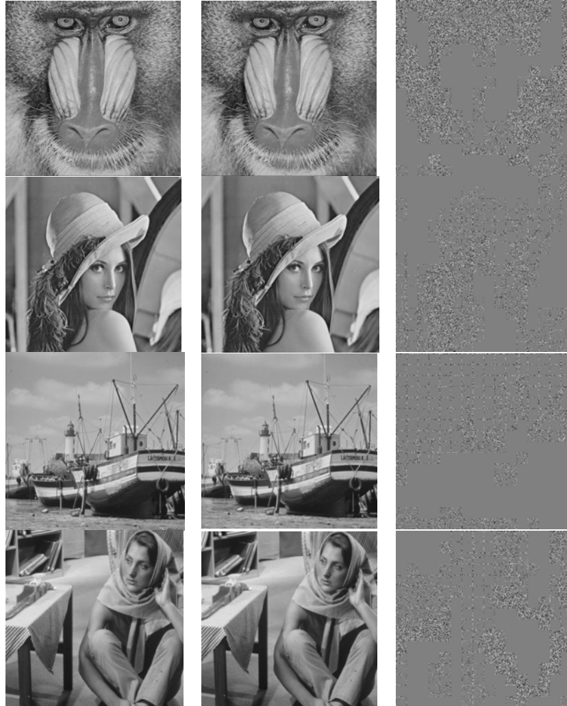
Fig. 3. Fingerprinted images, and their fingerprints (Enlarged), the number of Marks (M) =10, Repetition factor (R) =16, Block size = 32x32: (top) Baboon (PSNR: 40.69 dB), (second) Lena (PSNR: 44.07 dB), (third) Boat (PSNR: 45.45 dB), (bottom) Barbara (PSNR: 42.72 dB)
