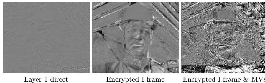
Fig. 6. The 50th P-frame of the Foreman sequence for different encryptions and attacks, no I-macroblocks are used (GOP with only P-frames).
