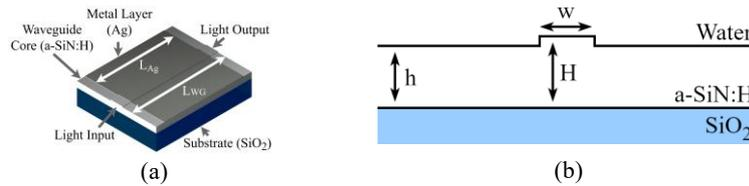
**Fig. 2.** Sensor design based on the rib waveguide. (a) Tridimensional model,  $L_{WG}$  and  $L_{Ag}$  represent waveguide and silver layer lengths, respectively. (b) Transversal section,  $w$  represents rib width,  $H$  rib height and  $h$  slab height.
