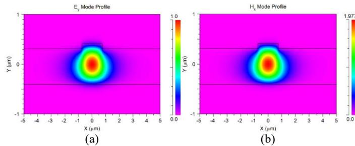
**Fig. 4.** Fundamental TM mode of the rib waveguide obtained in FEM simulation. (a) E<sub>y</sub> and (b) H<sub>x</sub> fields. Layers are delimited by black lines (from top to bottom, water, a-SiN:H and SiO<sub>2</sub>).
