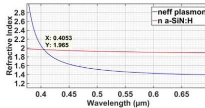
**Fig. 3.** Effective refractive index of the SPP (real component), represented in blue, refractive index of a-SiN:H with  $\text{Si}/\text{N} < 1$  (real component), represented in red. The intersection point shows an ideal SPP excitation wavelength of 405 nm and a refractive index of 1.965.
