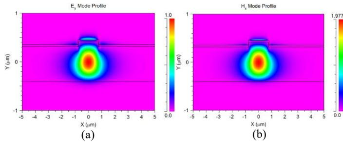
**Fig. 5.** FEM simulation results of the coupling between the fundamental TM mode and the SPP. (a) E<sub>y</sub> and (b) H<sub>x</sub> fields. Layers are delimited by black lines (from top to bottom, water, silver, a-SiN:H and SiO<sub>2</sub>).
