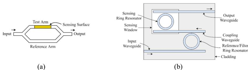
**Fig. 1.** Top view of two photonic sensor configurations (simplified). (a) Mach-Zehnder Interferometer (MZI) implementation based on waveguides, comprising Y-junction splitter and combiner. (b) An example of ring resonator topology, the Vernier-cascade sensor [22], this configuration comprises three waveguides and two ring resonators, the filter ring resonator and input waveguide are totally covered by the cladding.
