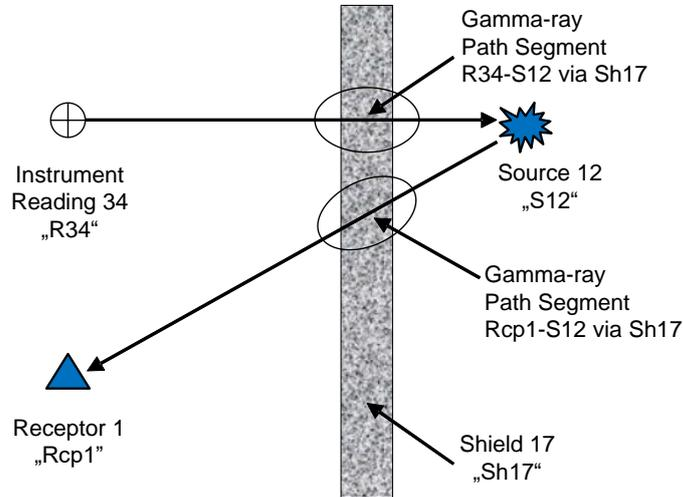
**Fig. 2.** Scheme of the forecast calculation using the EPRI method with shielded radiation
