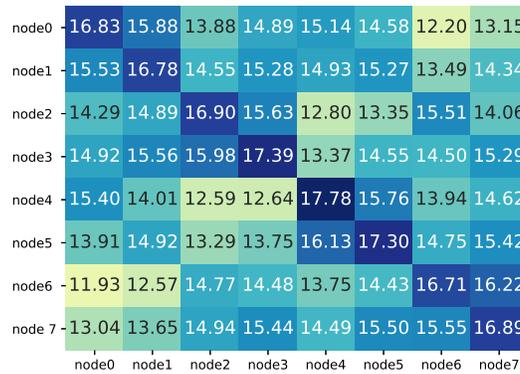
**Fig. 2.** STREAM triad bandwidth test on Phytium 2000+ .
