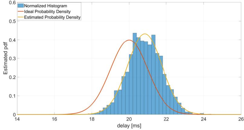
**Fig. 10.** Comparison of probability distributions: 2 GB RAM – 2 core CPU – Ubuntu Desktop OS
