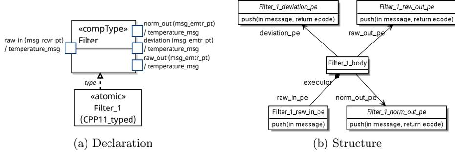
Fig. 1: Declaration and structure of UCM component `Filter_1`
