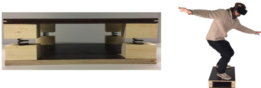
**Fig. 3.** The updated springboard iteration of the hoverboard device.
