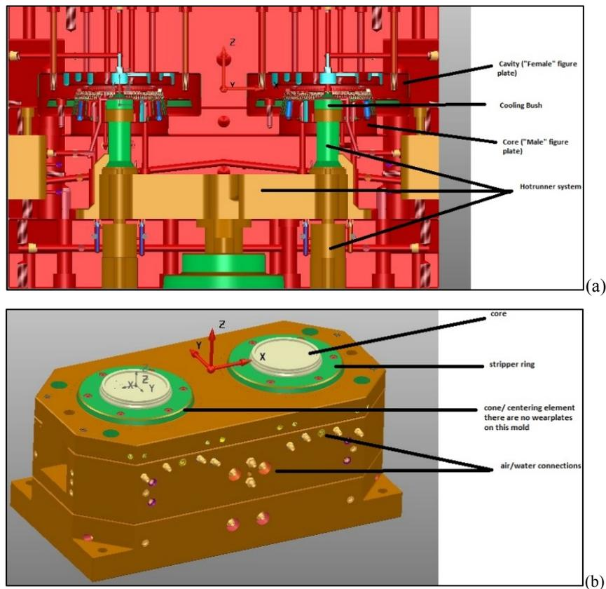
Fig. 2. “2 cavity, 1 liter Seal Lid” mold: General Section (a) and fixed side (b)
