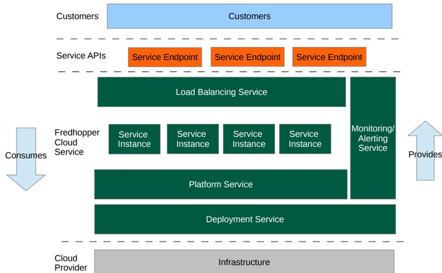
**Fig. 2.** The architecture of the Fredhopper Cloud Services
