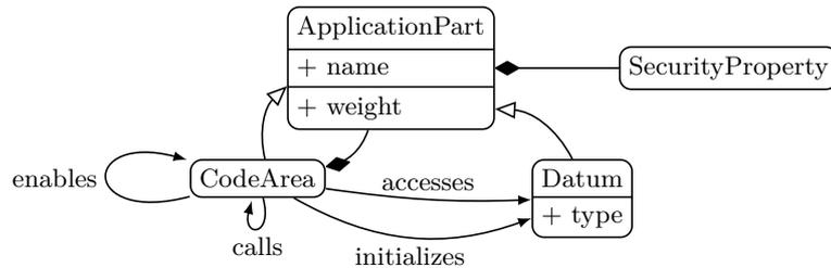
**Fig. 3.** UML class diagram of the application meta-model.
