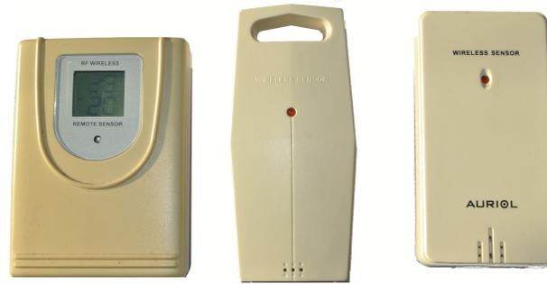
**Fig. 1.** The wireless sensors used for the evaluation (left-to right): H13716A-TX, Z31130-TX and Z31915-TX
