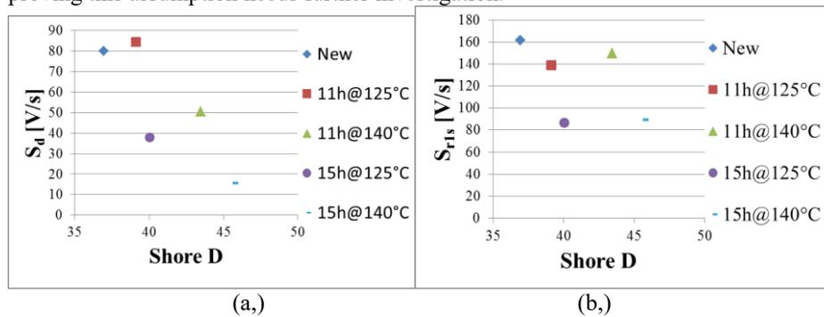
Fig. 5. Slope of decay voltage (S<sub>d</sub>) versus Shore D hardness (a,) Slope of return voltage after 1 s shorting time (S<sub>r1s</sub>) versus Shore D hardness (b,)
