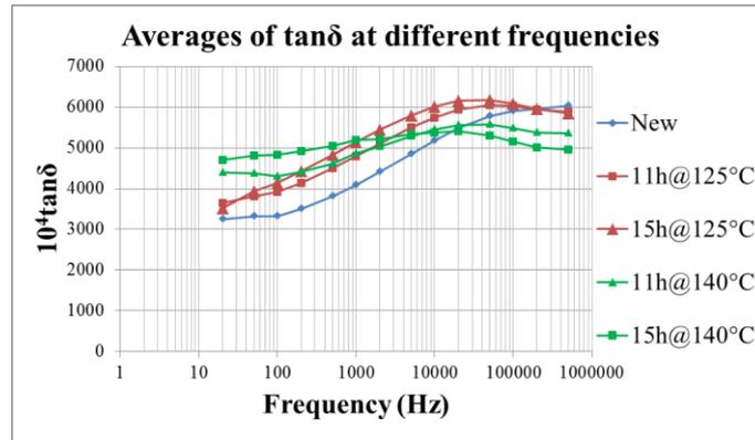
Fig. 3.  $\tan \delta$  as the function of frequency
