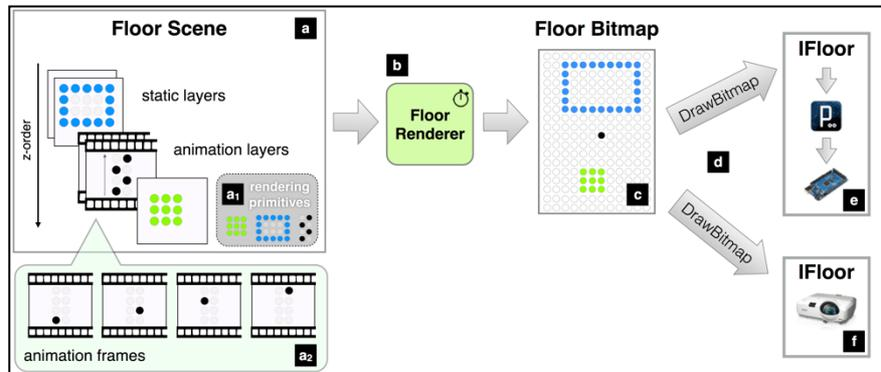
**Fig. 9.** The Proxemic Flow rendering pipeline: Visualizations on the floor display are abstracted in a floor scene (a). This floor scene is processed by the floor renderer (b), resulting in (c) a floor bitmap (an abstraction of a floor display update) that is sent over the network to the connected floor displays that implement the IFloor interface (d). We also implemented a projected floor display (f).
