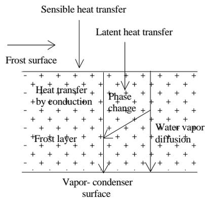
**Fig. 3.** The formation process of the frost
