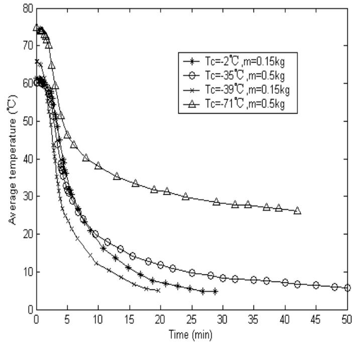
**Fig. 2.** Effect of temperature of vapour condenser on cooling rate during vacuum cooling
