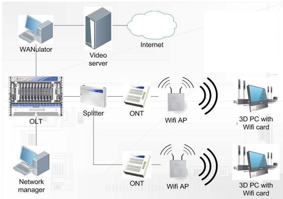
**Figure 1** The GPON-based + WiFi sub-networks topology
