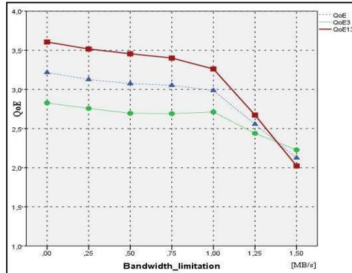
**Figure 3** QoE degradation based on bandwidth limitation
