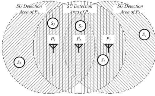
Fig. 1. SU detection area of three PUs.
