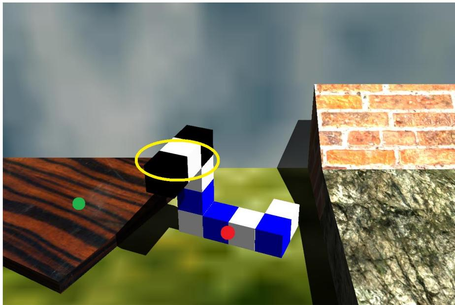
**Fig. 6.** In this example the Shepard-Metzler object is mated with the wooden floor to the left. If the user taps the object at the red dot and then taps the floor at the green dot, a naïve mating operation would result in the circled yellow part of the object disappearing into the wooden floor.
