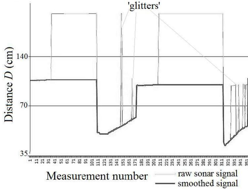
Fig. 2. Raw sonar measurements and real objects
