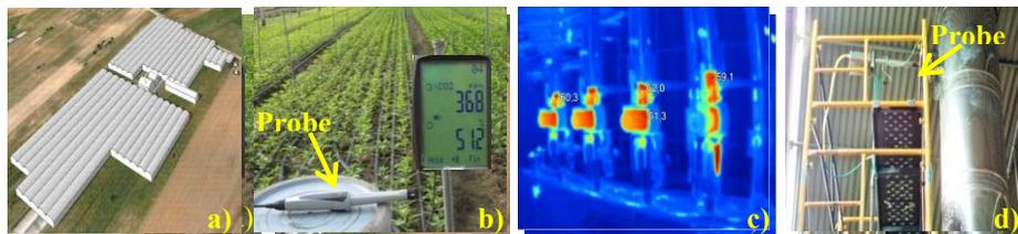
**Fig. 2.** Data collection in greenhouse: a) Greenhouses overview; b) Temperature, humidity, CO<sub>2</sub>; c) Thermographic images of hot water pumps; d) Gaseous emission probe.
