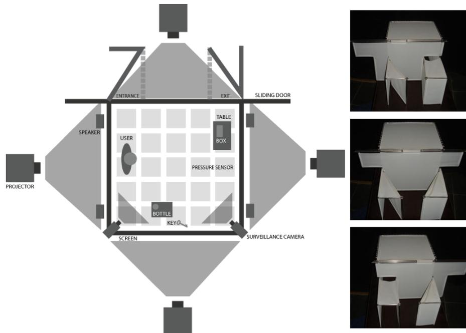
**Fig. 1.** Overview of “Eat me, drink me” stage. (a) left, the schematic overview of the physical setting (b) right, the scale model of the CAVE, from top to bottom: (1) the entrance is opened, (2) the entrance and exit are closed, (3) the exit is opened
