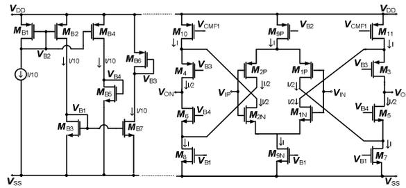
Fig. 1. Proposed inverter-based single-stage folded-cascode OTA (FCA).
