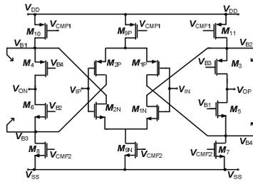
Fig. 3. Proposed inverter-based single-stage FCA employing RFF and self-biasing (SB).
