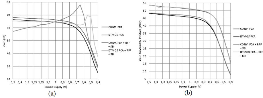
**Figs. 5.** Simulated DC gain (a) and Simulated gain-bandwidth product (b) for different positive ( $V_{DD}$ ) supply voltage conditions (ranging from 0.4 V to 1.5 V), for the conventional FCA (Fig. 1) and for the modified amplifiers shown in Fig. 2, Fig. 3 and Fig. 4.
