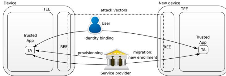
Fig. 1: The life cycle of a TEE service
