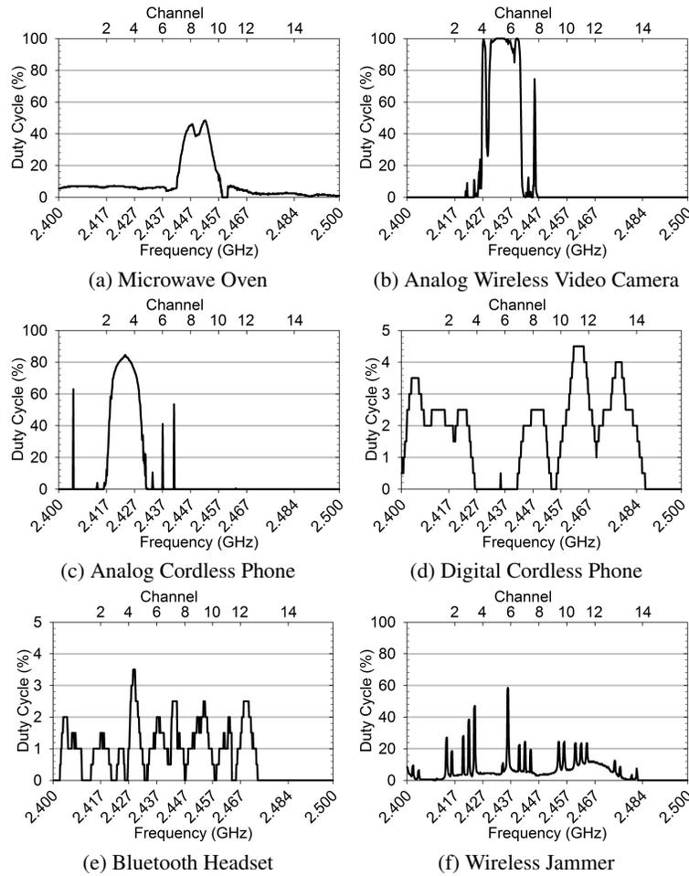
**Fig. 4.** Duty cycle analysis for six non-Wi-Fi devices
