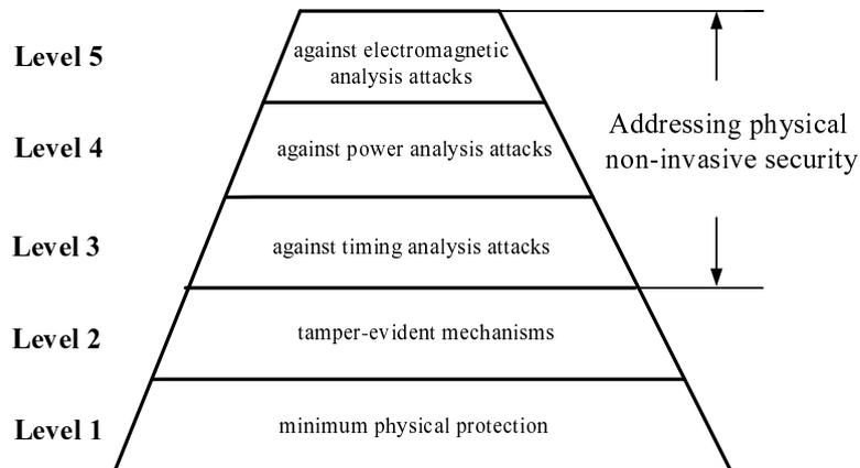
**Fig. 1.** Physical non-invasive security addressed by FIPS 140-3
