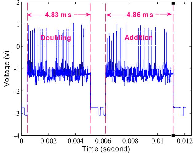
**Fig. 8.** Indistinguishable power trace of doubling and addition on device B
