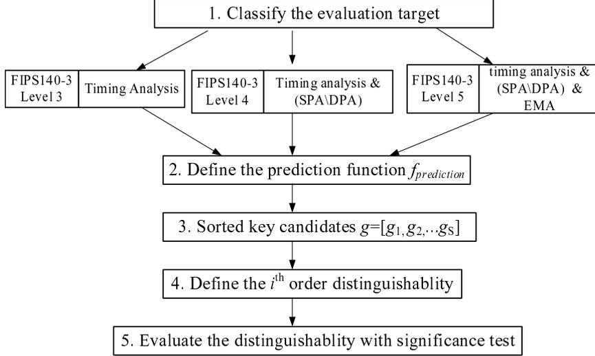
**Fig. 2.** Quantitative evaluation procedure for physical non-invasive security
