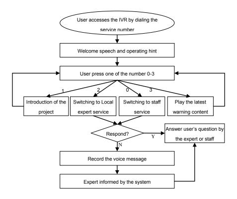
Fig. 1 Tthe flowchart IVR in the system
