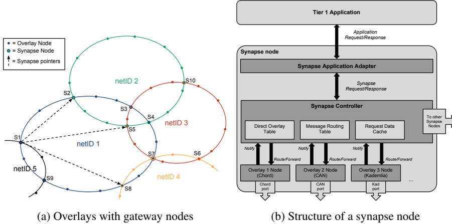
Fig. 1: Inter-overlay topologies and structure of synapse nodes
