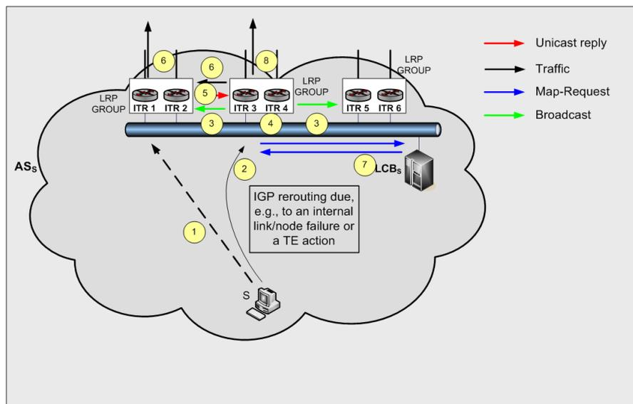
Fig. 6 ITR has no mapping from EID-to-RLOC
