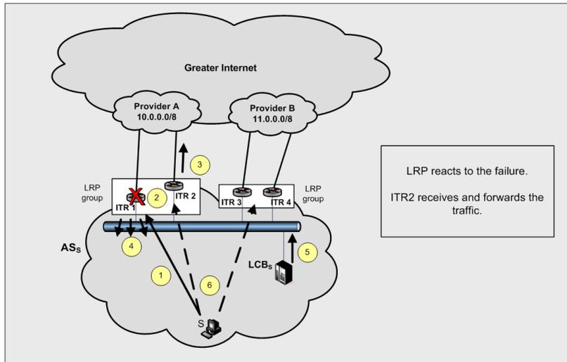
Fig. 5 ITR Failure
