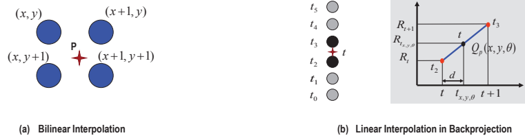
Fig. 2. Interpolation in CT Backprojection
