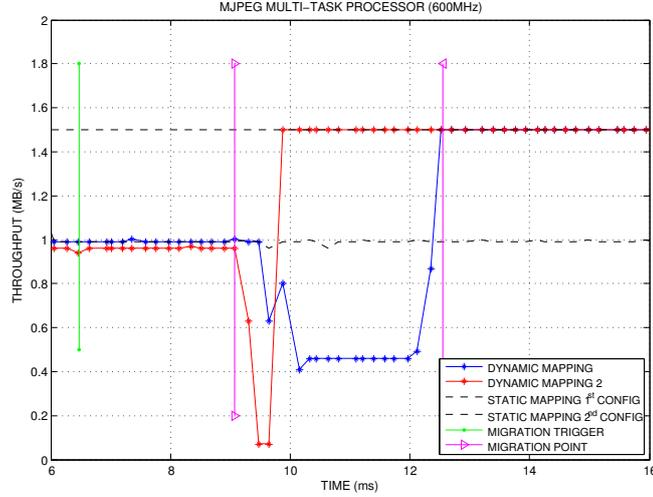
**Fig. 14.** Throughput of MJPEG for each case
