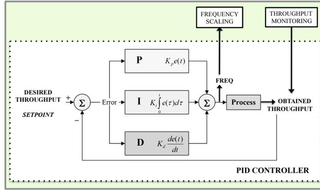
Fig. 2. PID Controller
