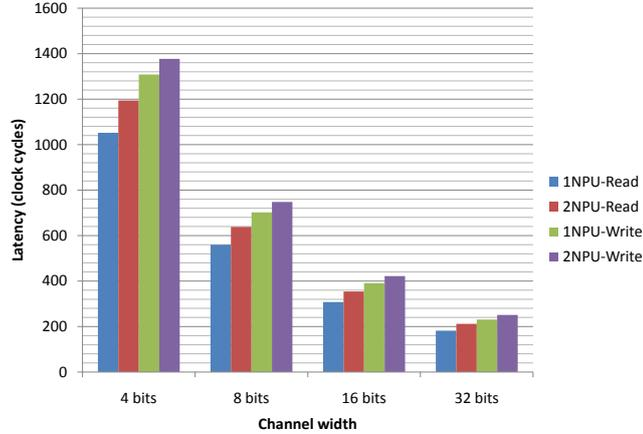
**Fig. 19.** Time to memory access in clock cycles
