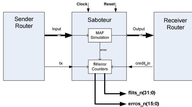
Figure 5 – Saboteur located between two routers.
