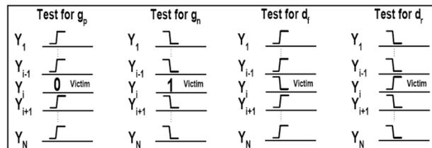
**Figure 4 - Required transitions for MAF model [1].**
