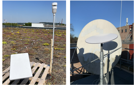
Fig. 2: Our measurement setups. In this picture, the Froggit DP2000 weather station can be seen placed directly next to the Starlink dish.
