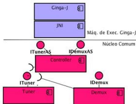
**Figure 5 - Ginga-J Execution Layer and Common Core integration**
