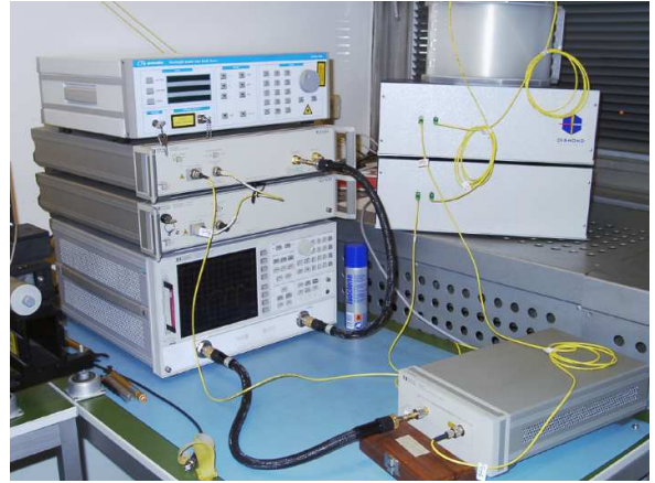
Fig.17. Photograph of the experimental setup for the fundamental RF level measurements
