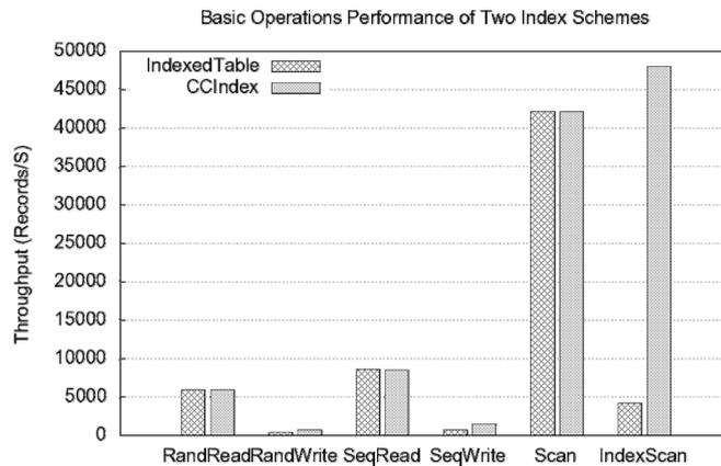
**Fig. 3.** Basic Operation Performance of Two Index Schemes. CCIndex throughput is 11.4 times of IndexTable's in *IndexScan* operation. CCIndex random *write* and sequential *write* operations is 54.9% and 121.4% better than that of IndexTable.
