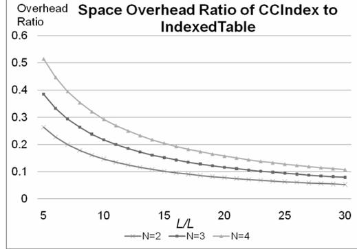
**Fig. 2.** The space overhead ratio of CCIndex to IndexedTable. The overhead ratio drops significantly as the  $L/L_n$  increases and the  $N$  decreases. If  $N$  changes from 2 to 4 and the  $L/L_n$  changes from 10 to 30, then the overhead changes from 5.3% to 29.3%.
