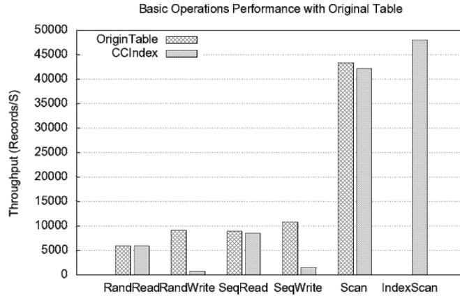
**Fig. 4.** Basic Operation Performance with Original Table. CCIndex *IndexScan* throughput is 10.9% more than origin table. The *random write* and *sequential write* is significantly lower than the origin table due to the overhead to maintain index, which is a common issues for both index schemes.
