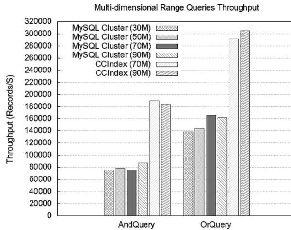
**Fig. 6.** Multi-dimensional range queries throughput for multiple clients. MySQL Cluster performance is stable when the data sets increases from 30 million to 90 million records. With the 90 million records, CCIndex AndQuery and OrQuery throughput is 2.1 and 1.9 times of the memory-based parallel database MySQL Cluster.
