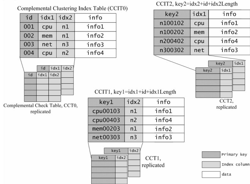
**Fig. 1.** Data layout of CCIndex. For a logical table has *id* as the primary key with two index columns *idx1* and *idx2*, CCIndex creates another two CCIT tables each for a index column and reorganizes the rows in the order of this column. CCIndex creates replicated CCTs for fast data recovery.
