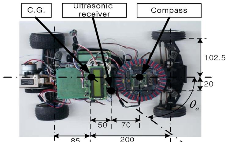
**Fig. 4.** Configuration of 1/10 vehicle (unit: mm)
