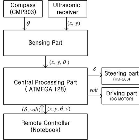
**Fig. 5.** Configuration of hardware
