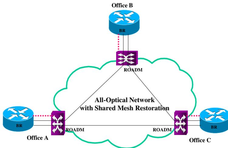
**Figure 4: Integrated IP-over-Optical Layer Restoration**
