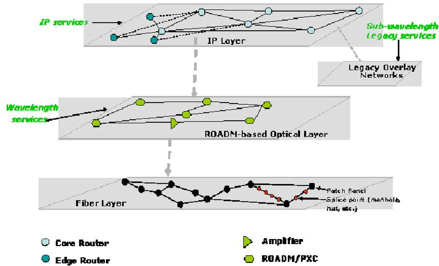
Figure 1: IP over Reconfigurable All-Optical Network Architecture
