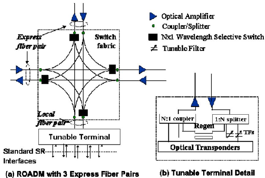
Figure 2: A Broadcast-and-Select ROADM Architecture
