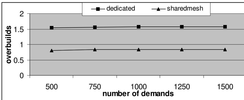
Figure 6: Restoration Overbuild Comparison with a Fixed Double Failure Ratio (5%)
