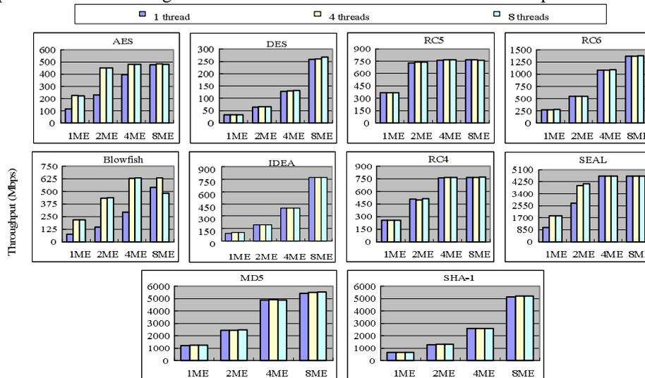
Fig. 5. Throughput of selected algorithms with varying number of threads and MEs
