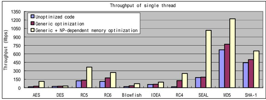
**Fig. 3.** Single thread performance with different optimization principles
