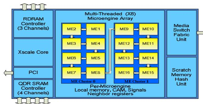
**Fig. 1.** The hardware architecture of Intel IXP2800
