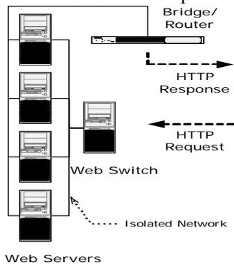
Fig. 1. Web Server Cluster with Isolated System Network
