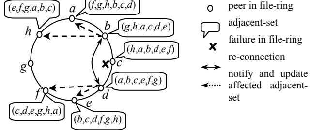
**Fig. 3.** Maintaining file-ring connectivity
