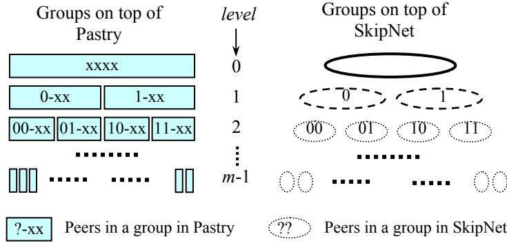
**Fig. 1.** Partition on top of Pastry and SkipNet.
