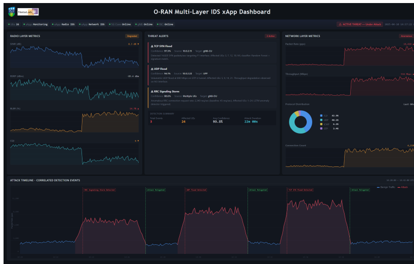
Fig. 2. O-RAN multi-layer IDS dashboard showing radio-layer degradation, detected threat alerts, network-layer anomalies, and a correlated attack timeline.
