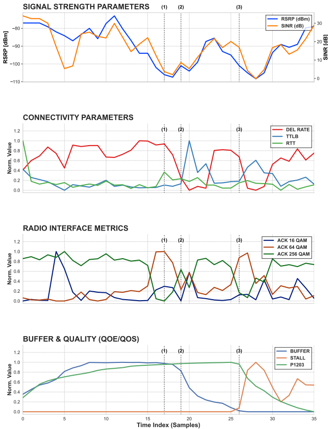
Fig. 2: Cross-metric correlation analysis. The top plot illustrates absolute signal strength values (RSRP, SINR), while the bottom panels show normalized relationships between connection quality (Delivery Rate, TTLB, RTT), Buffer state, and QoE metrics (Stall, ITU-T P.1203 [15]). [QoS 5QI = default, W = 10 ]
