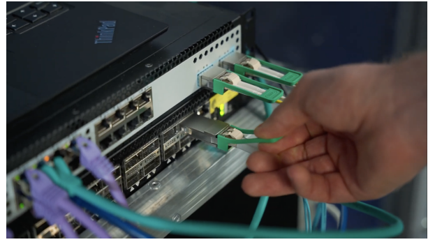
Fig. 4. Unplugging the hardware-based UPF.
